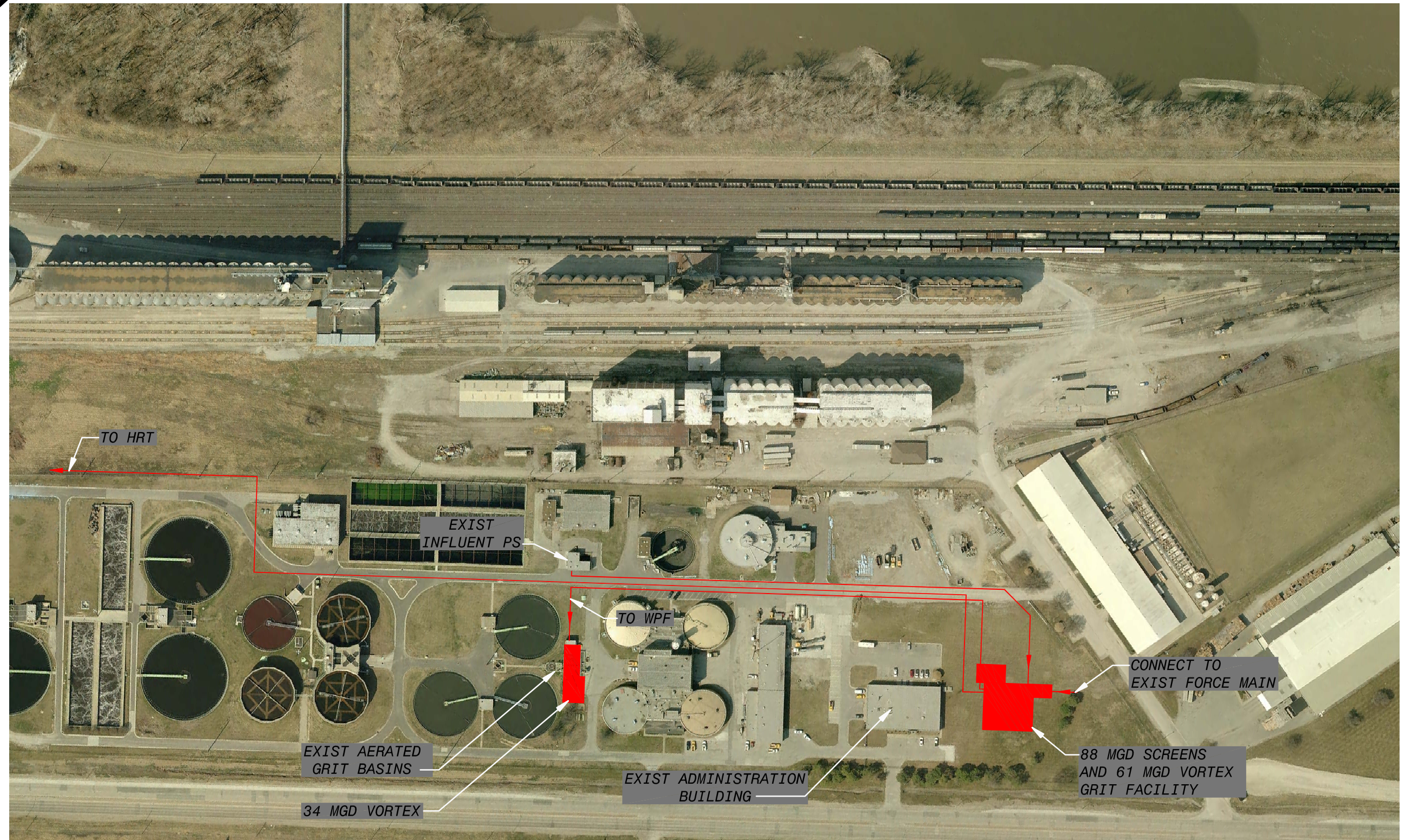
ST. JOSEPH, MISSOURI FACILITIES PLAN PN 163509 ALTERNATIVE 3A-1 SCREENING FOR 88 MGD, GRIT REMOVAL FOR 34 MGD, AND GRIT REMOVAL FOR 61 MGD - VORTEX BLACK & VEATCH DECEMBER 2009 FIGURE 22
