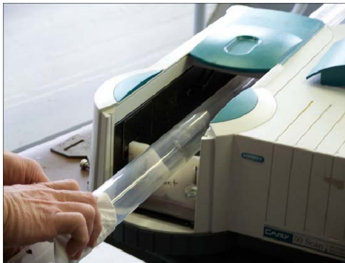
Figure 8 Sleeve Measured for UVT in Varian Cary 50 UV/Visible Spectrophotometer
